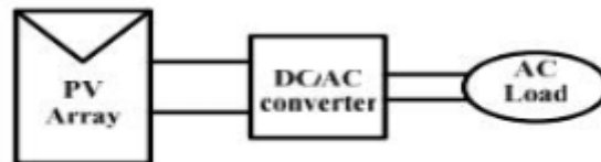
Fig. 11: Block diagram representation of Photovoltaic system
